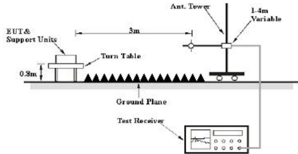
The radiated emission tests below 1GHz were performed in 10 meters, above 1GHz were performed in the 3 meters, using the setup accordance with the CISPR 16-1-1:2010+A1:2010, CISPR 16-1-4:2010, CISPR 16-2-3:2010. The specification used was EN 55032 Class B limits.
