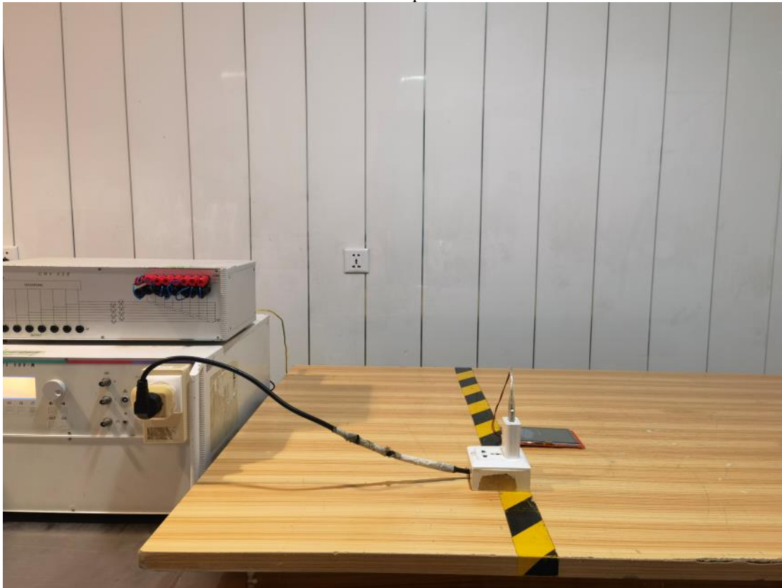
AC Port Test Setup Photo View
