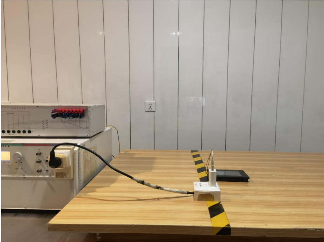
AC Port Test Setup Photo View
