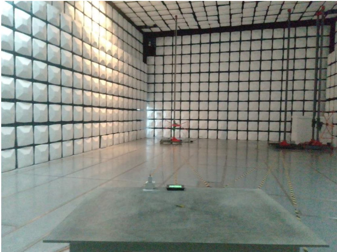
RE Below 1G front View
