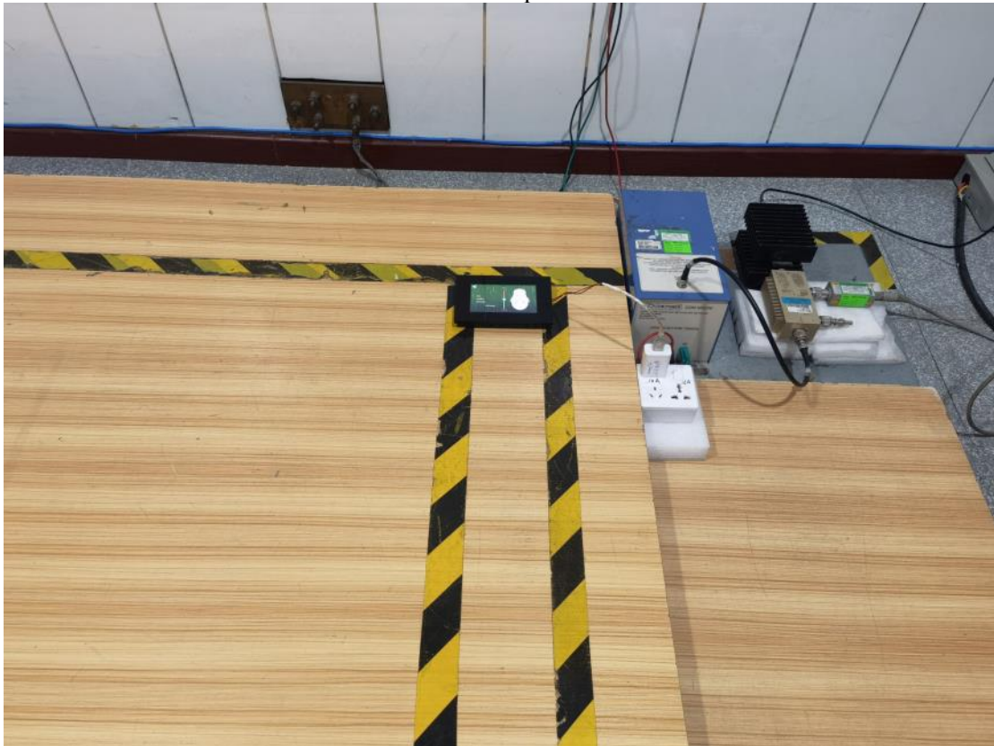
AC Port Test Setup Photo View
