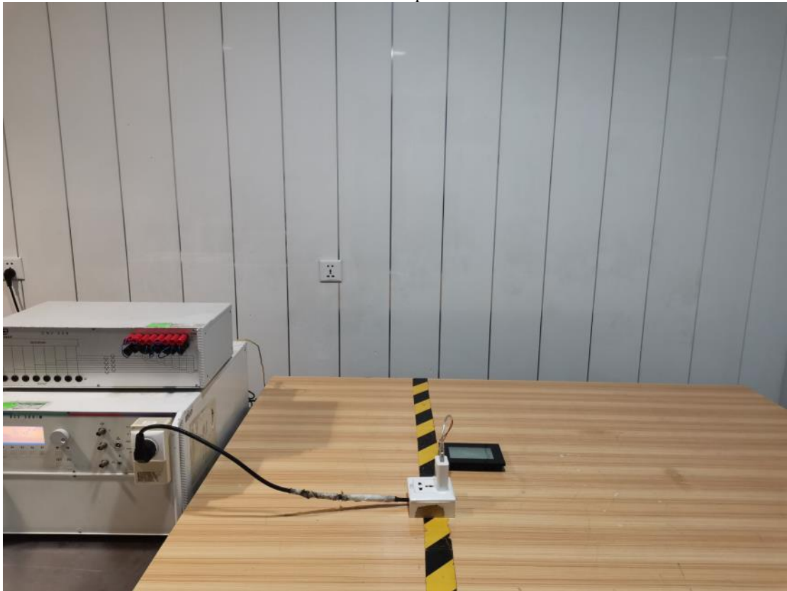
AC Port Test Setup Photo View
